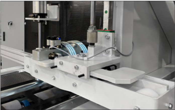
Positioning reading system with double wheels for special workpiece without edged.
